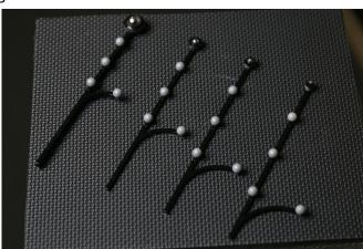
Fig. 1. **4x4 Grid of Magnetometers and Tracking Wands with Magnets.** (A) A 4x4 magnetometer array was created using a 3d-printed structure with reflective markers for tracking. (B) Each magnet was attached north-pole-up to a unique 3d-printed wand with reflective markers for tracking.
